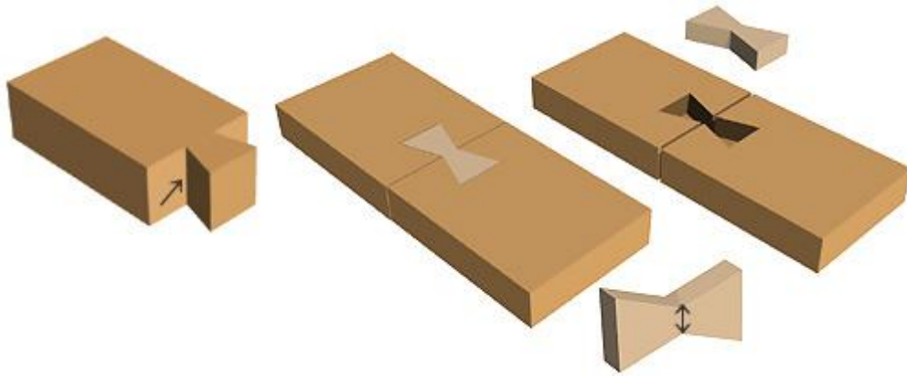
arikubi spline * chigiritsugi 千切継 : dovetail neck narrow west part
